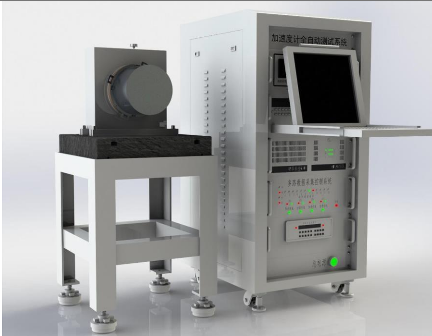
Repeatability test equipment
