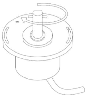
Figure 1.1 The direction of the arrow is the clockwise rotation direction of the sensor.
